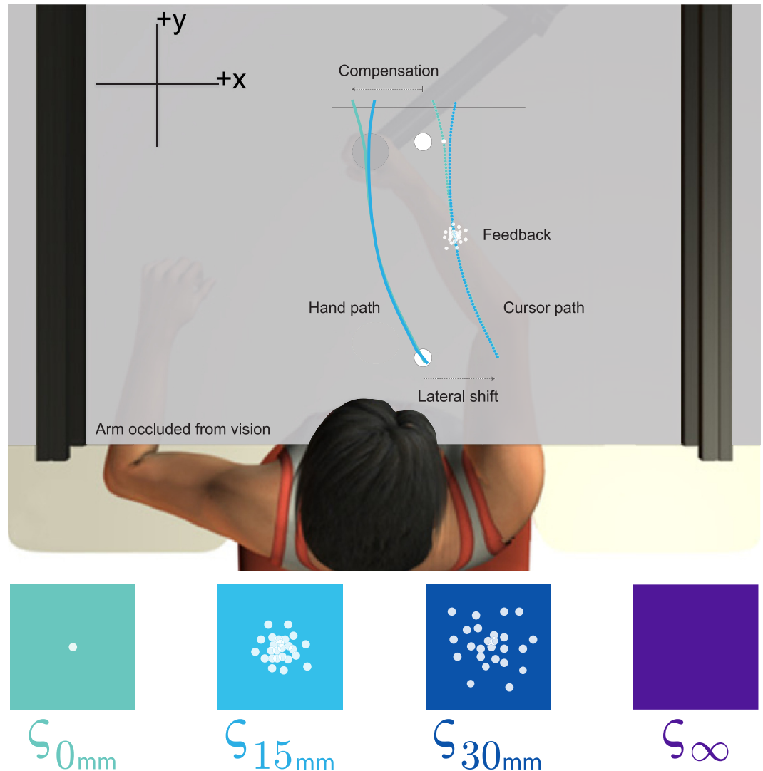
Fig 1. Experiments 1 and 2: Participants held the handle of a robotic arm with their right hand. A semi-silvered mirror reflected the image (visual targets, visual feedback) from an LCD screen (not shown) onto a horizontal plane aligned with the shoulder. Participants made forward reaches from a home position, attempted to move through a visual target and stopped once their hand passed over a horizontal line that disappeared when crossed. Error (visual) feedback and reinforcement (target expands, pleasant sound and monetary reward) feedback was laterally shifted relative to true hand position. The magnitude of any particular lateral shift was drawn from a skewed probability distribution. Participants had to compensate for the lateral shifts to hit the target. Compensation represents how laterally displaced their hand was relative to the displayed target. Experiment 1: Laterally shifted error feedback was flashed halfway through each reach as a single dot ( \zeta_{0mm} ), a medium cloud of dots ( \zeta_{15mm} ), a large cloud of dots ( \zeta_{30mm} ), or withheld ( \zeta_{\infty} ). The cursor and hand (not visible) paths shown above illustrate compensation that depended on the amount of visual uncertainty ( \zeta_{0mm} and \zeta_{15mm} conditions shown). In the single dot ( \zeta_{0mm} ) condition, participants received additional feedback (error or error + reinforcement) at the target. Experiment 2: Participants were provided with error feedback and or reinforcement feedback only at the target.
