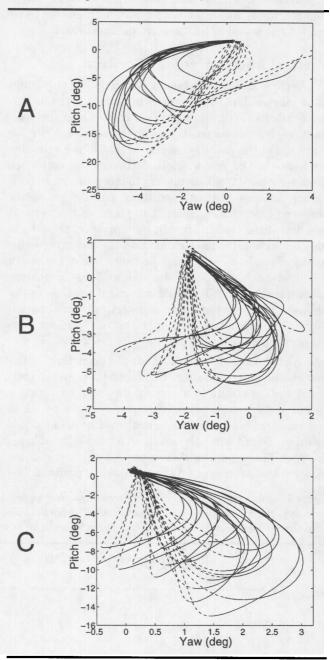
shows two examples that suggest that yaw and pitch orientations in speech may vary independently. The figure shows sagittal plane jaw orientation (pitch) over the course of an opening movement plotted as a function of the yaw angle. The upper panel shows movements in which the relationship between yaw and pitch angles is reversed—the jaw rotates laterally in one direction during jaw opening for one of the movements shown in the figure and rotates laterally in the opposite direction
