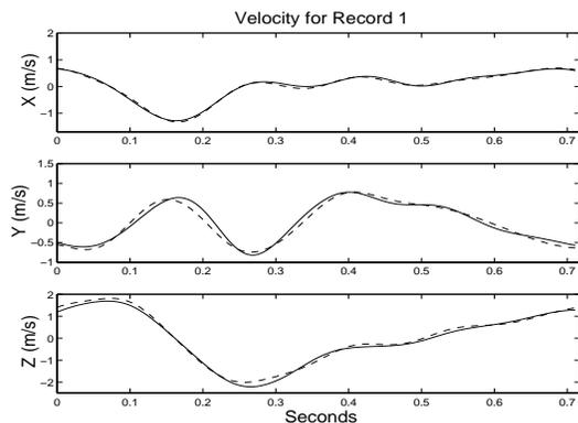
Figure 11: The actual velocity coordinate functions  $V_{ik}(t)$  are plotted as dashed lines, and the fit based on the homogeneous linear differential equation of order two is plotted as a solid line. The data are for the first record.
